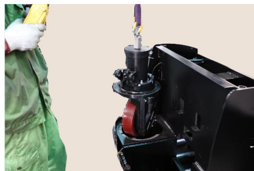
④ Rotate a certain angle and lift the drive wheel with a tool
